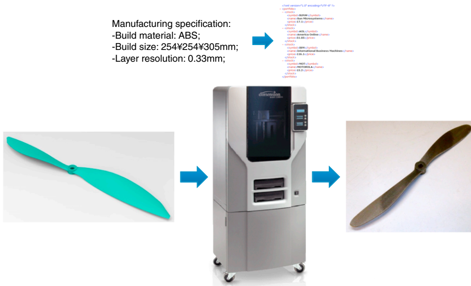
Fig. 11. Build the propeller of the drone using 3D printing [60].
